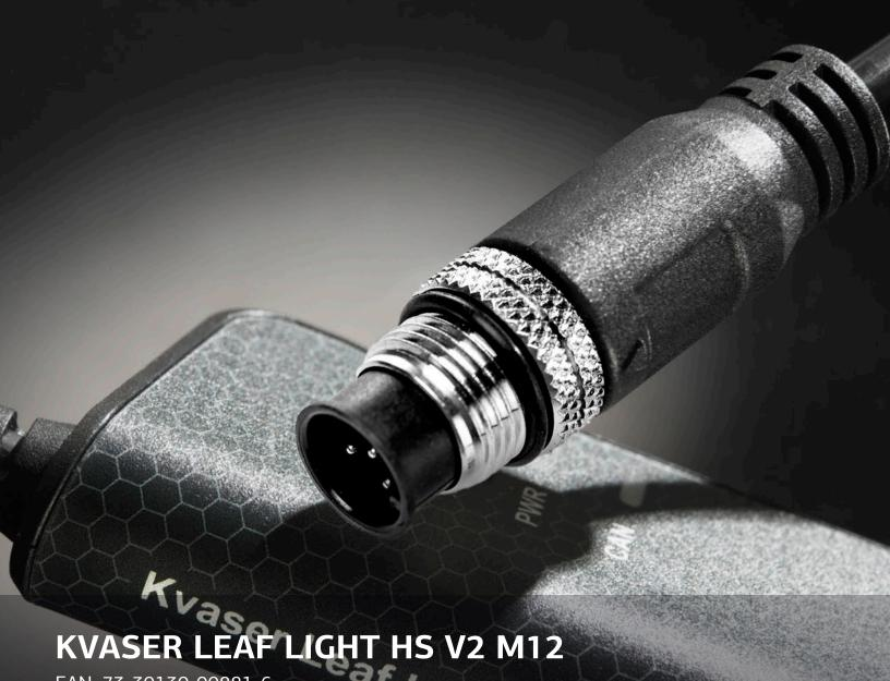
The The Leaf Light HS v2 M12 is the marine version of Kvaser's popular Leaf Light v2 interface. This device provides a simple way of connecting a PC with the on-board computer of a marine electronics system by means of its standard USB 2.0 connector and a 5-pin National Marine Electronics Association (NMEA) approved CAN connector. The Leaf Light HS v2 M12 is ideal for diagnosing NMEA 2000 bus issues, configuring and flashing NMEA 2000 bus nodes, monitoring NMEA 2000 bus traffic and load
