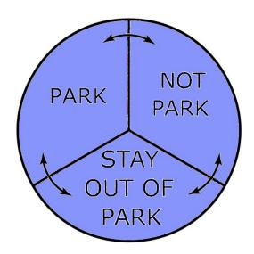
Switching to any of these modes can be achieved with the three buttons on the front of the IPM test module and appears on the LCD display. Along with displaying the current state based on the feedback sensors, the actual feedback signals are output on 4 BNC connectors for recording or viewing on an oscilloscope. The IPM test module comes with a wall plug power adaptor and custom cable sets are available.
